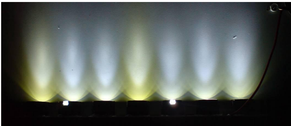
Figure 3. Color shift due to solvent penetrating inside the LED
